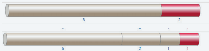
Figure 4: Two cutting patterns for a master roll of width 10".
